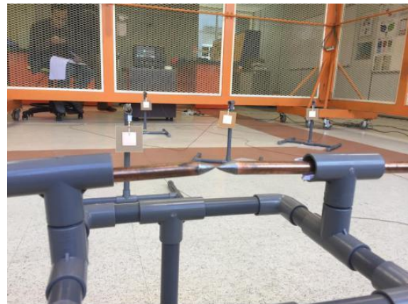
Figure 4. Laboratory arc generator experiment setup.
