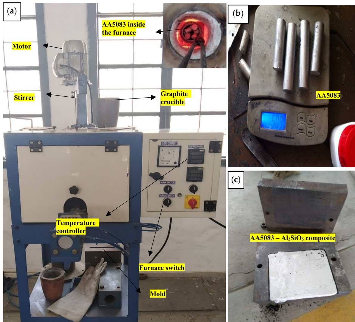
Figure 1. Casting equipment: (a) experimental compo-casting setup; (b) matrix material; (c) AA5083— \text{Al}_2\text{SiO}_5 compound.
