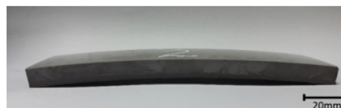
Fig. 5 – Curved thin fly ash geopolymer synthesised with S/L ratio of 1.5.
