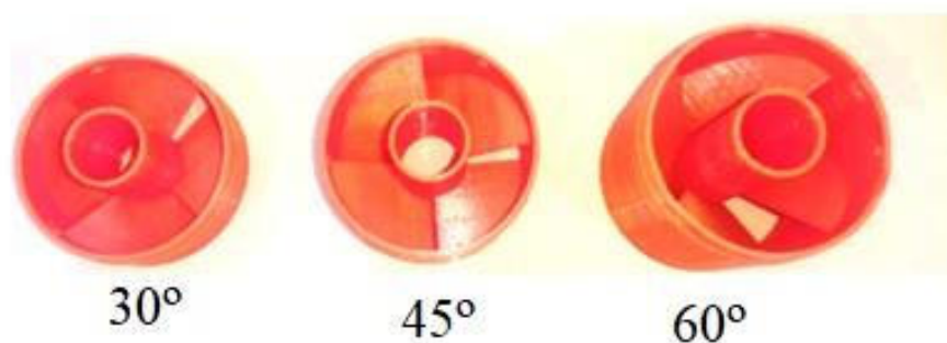
Figure 5. The fan blade angles of the FBHSSR design model.
