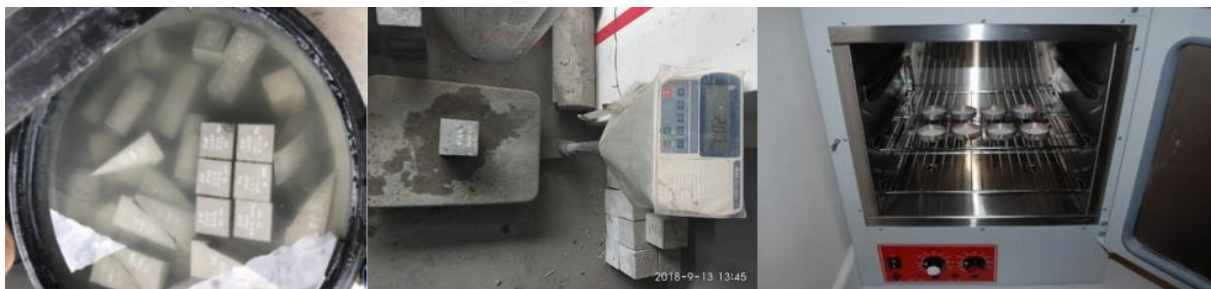
Figure 2. Water absorption test process.
