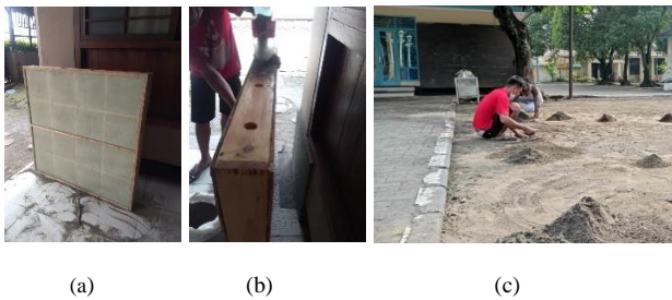
Figure 2. (a) The test material module is a wooden frame; (b) sand is inserted into the test material module frame; and (c) the test material sand is obtained from the courtyard of the Great Mosque of Surakarta
