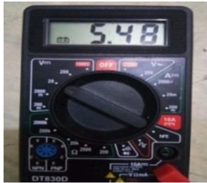
Figure 9. PIR Sensor Voltage Measurement Results
