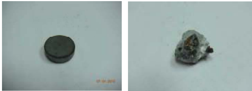
Figure 1: Appearance of sample before and after arc melting
