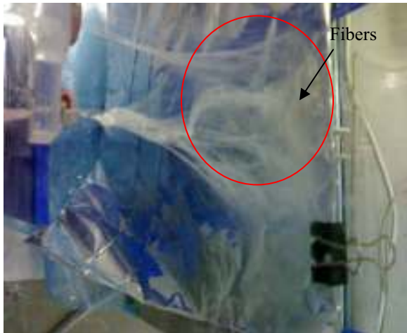
Figure 1: The fiber formation during electrospinning process
