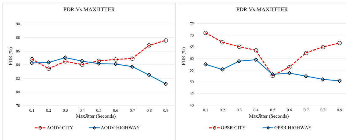
Figure 4. PDR comparison between VANET scenarios and MaxJitter.
