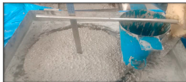
Fig. 2. Slump cone setup as per BIS 1199.
