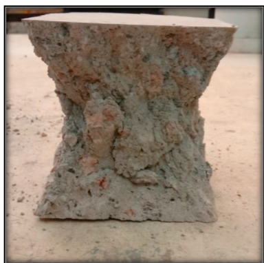
Fig. 11. Failure of specimen after compressive destruction.
