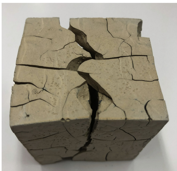
Fig. 11 – Major cracking after two-steps of sintering of sintered kaolin-GGBS geopolymer due to inadequate curing condition.
