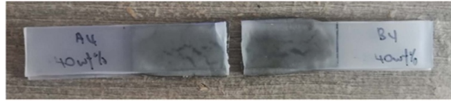
Figure 14. Photograph of 40 wt% welded sample after being subjected to three-point bending test.
