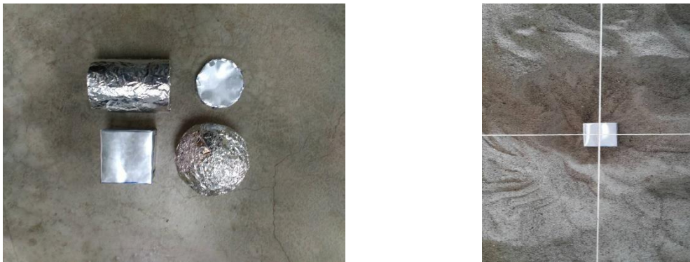
Figure 5. Example of samples used in the experiment (left) and sample buried in the testbed (right).
