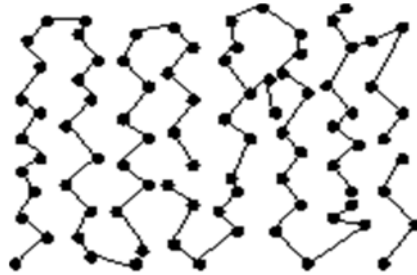
Figure 2.2: Illustrative structure representative of HDPE (Durmus et al, 2007).
