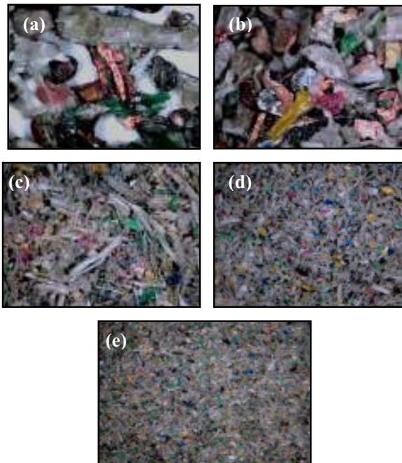
Figure 1: Distribution of comminution fines waste PCBs in five size ranges fraction
