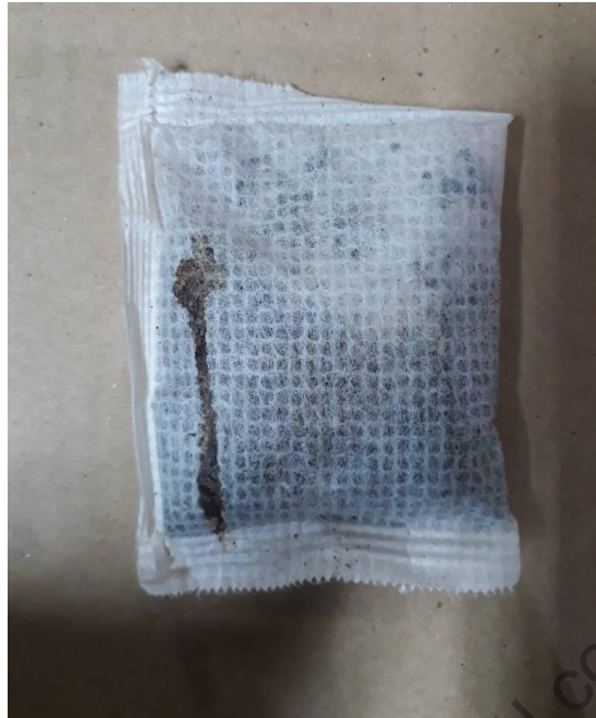
Figure 1.7 : Black Line Defect
