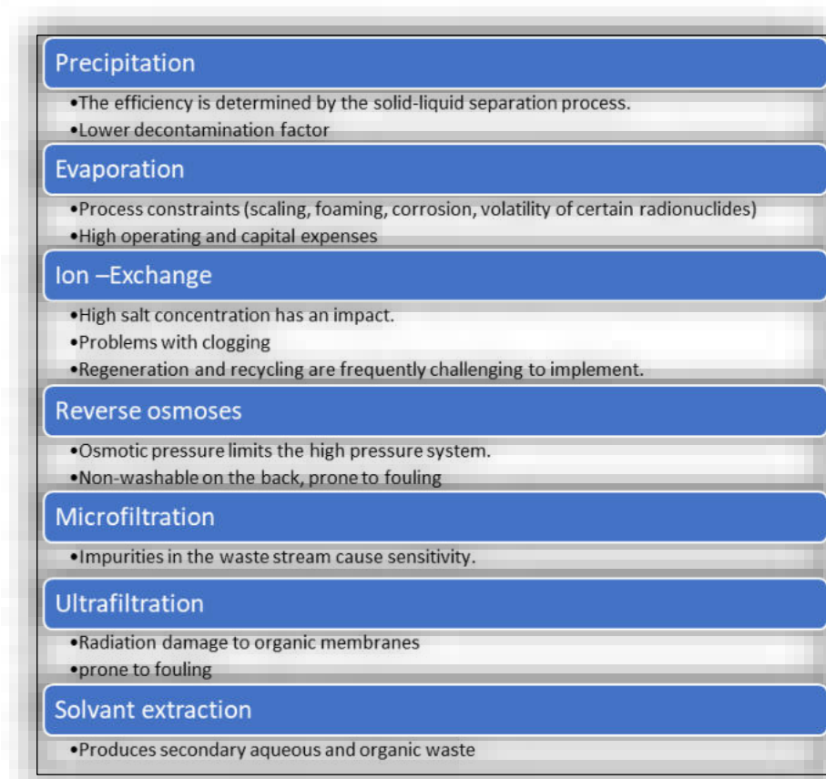
Figure 5. The limitations of various aqueous liquid treatment solutions.
