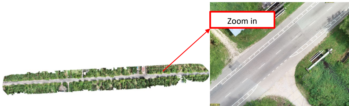
Figure 3. Orthomosaic images produced using Pix4DMapper.
