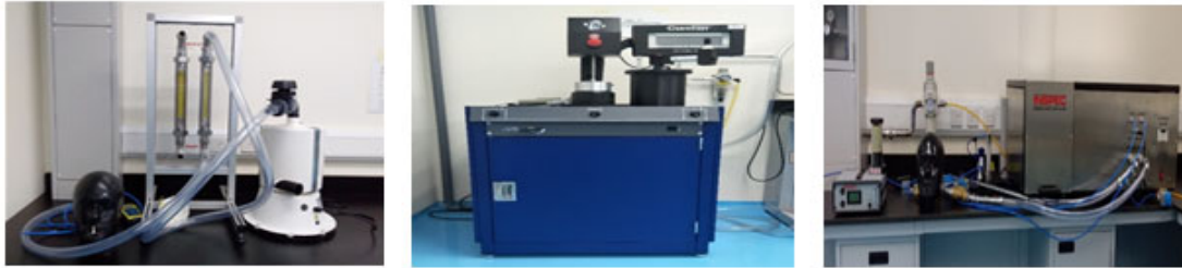
Figure 5. Testing equipment breathing resistance, high flow automated filter tester and CO 2 of Inhalation air
