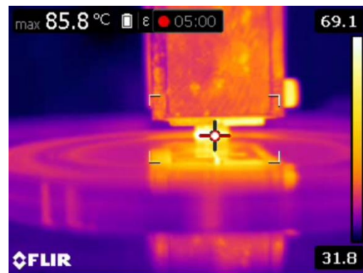
Figure 8. Temperature of the pure aluminium pin at 50 N loads at 5 min.
