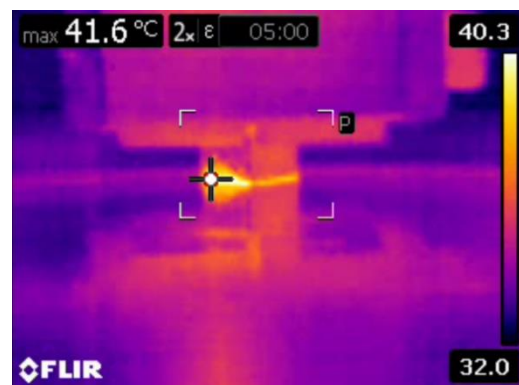
Figure 16. Temperature of the hybrid composite pin at 50 N loads at 5 min.
