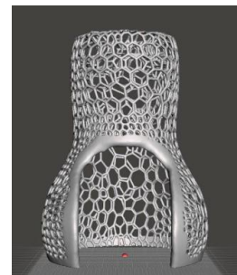
Figure 9. Voronoi pattern of optimized socket (Back view).
