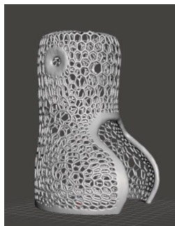
Figure 7. Voronoi pattern of optimized socket (Side view).
