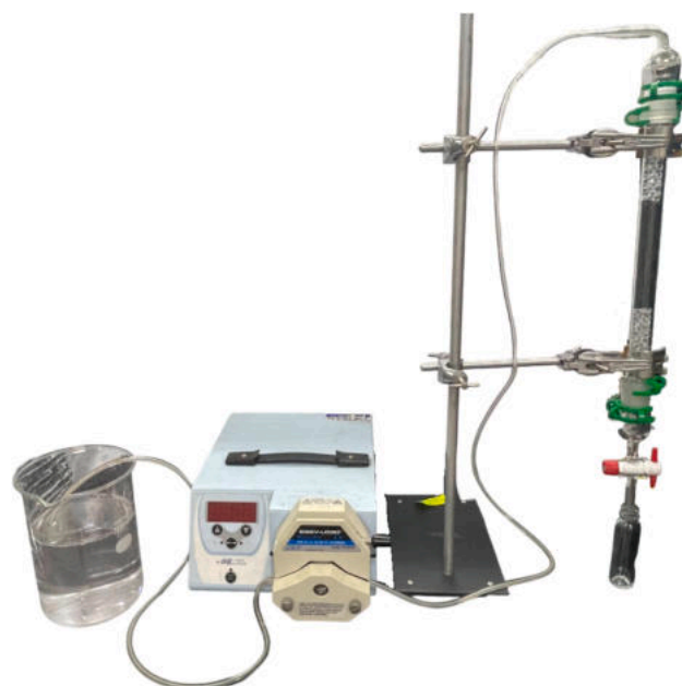
Fig. 1. Experimental setup of MP and NP removal study.
